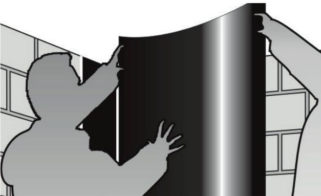
Overlap the KÖSTER KSK Membrane by at least 10 cm onto the piece of membrane applied in the corner.
